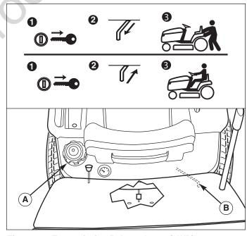
Figure 2.1. Transmission Release Lever (2WD)
